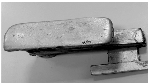
Figure 2: Bottom gating system
