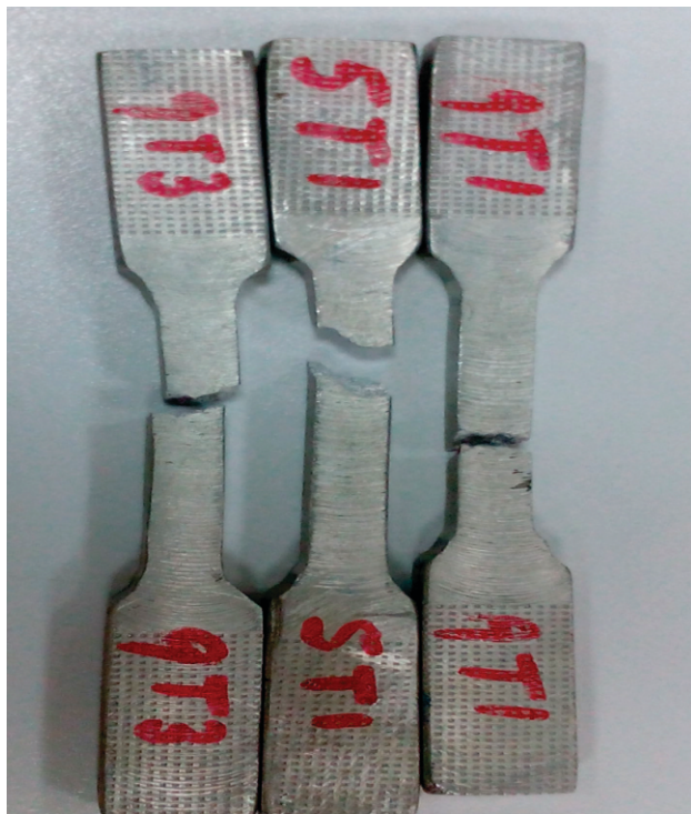
Figure 6: Broken Samples after Testing
