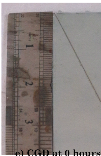
Figure 7: Photographic images Zinc Electroplated (ZnE), Cold Galvanized Brushed (CGB) and Cold Galvanized Dipped (CGD) at 0 & 500hrs.
