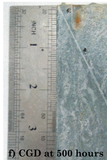
Figure 7: Photographic images Zinc Electroplated (ZnE), Cold Galvanized Brushed (CGB) and Cold Galvanized Dipped (CGD) at 0 & 500hrs.
