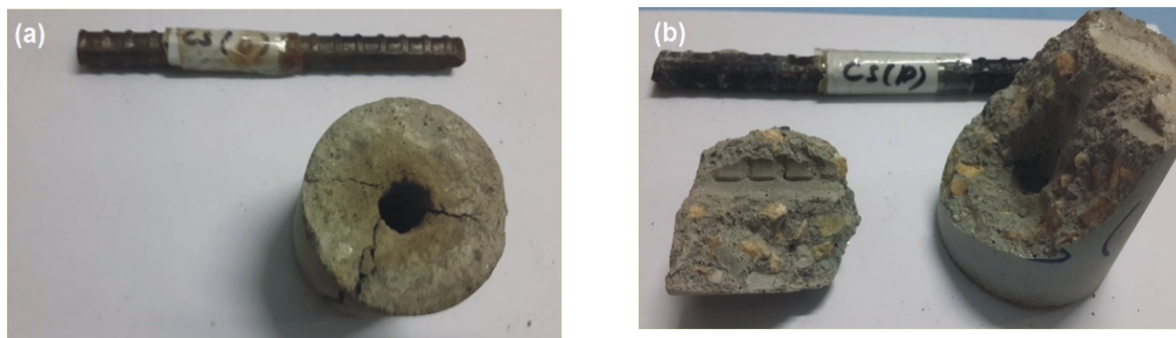
Figure 9: Failure of concrete specimen after pull out test
