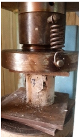
Figure 4: Concrete specimen during compressional test
