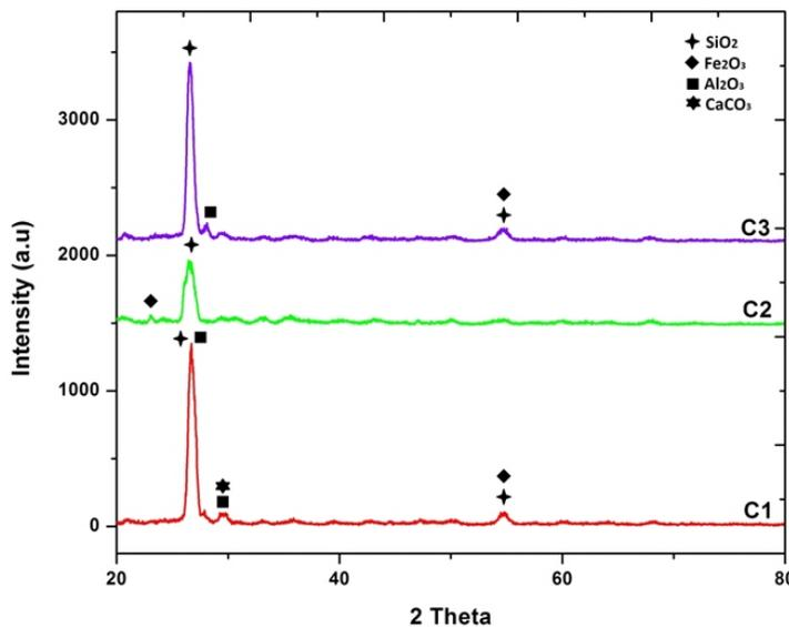
**Figure 6:** XRD pattern of developed foundry refractory coating.
