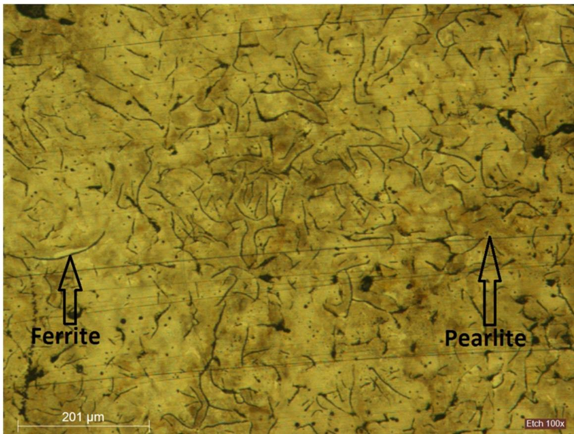
**Figure 9:** Microstructure Analysis of the Grade 14 at 100x (Etched in 2% Nital).
