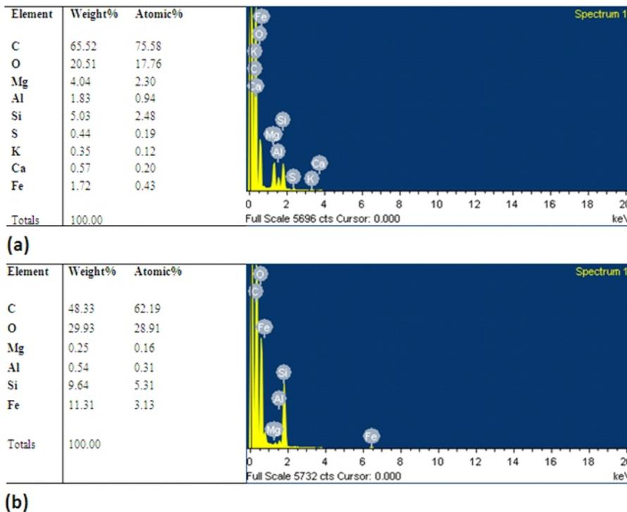
**Figure 3:** EDS analysis of dry refractory coating (a) and (b).
