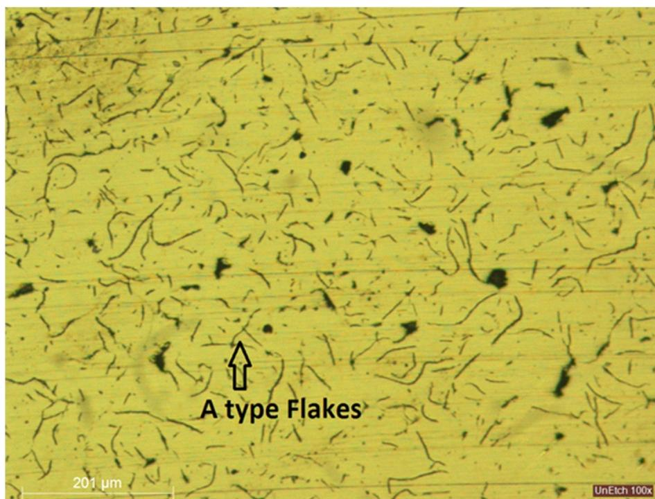
**Figure 8:** Microstructure Analysis of the Grade 14 at 100x (Unetch).
