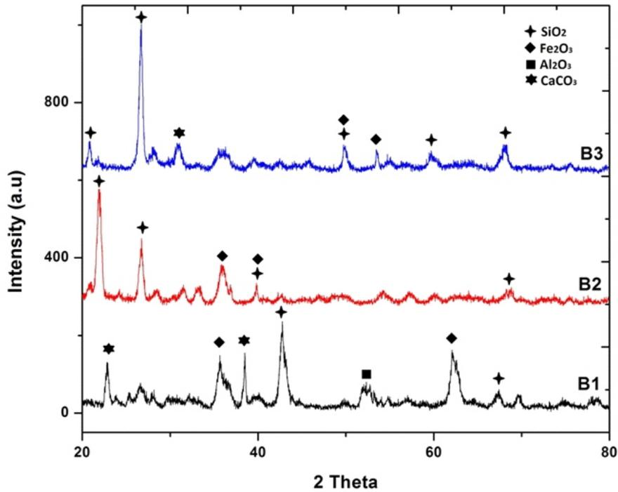
**Figure 2:** XRD pattern of the heat treated (1000°C) foundry refractory coating
