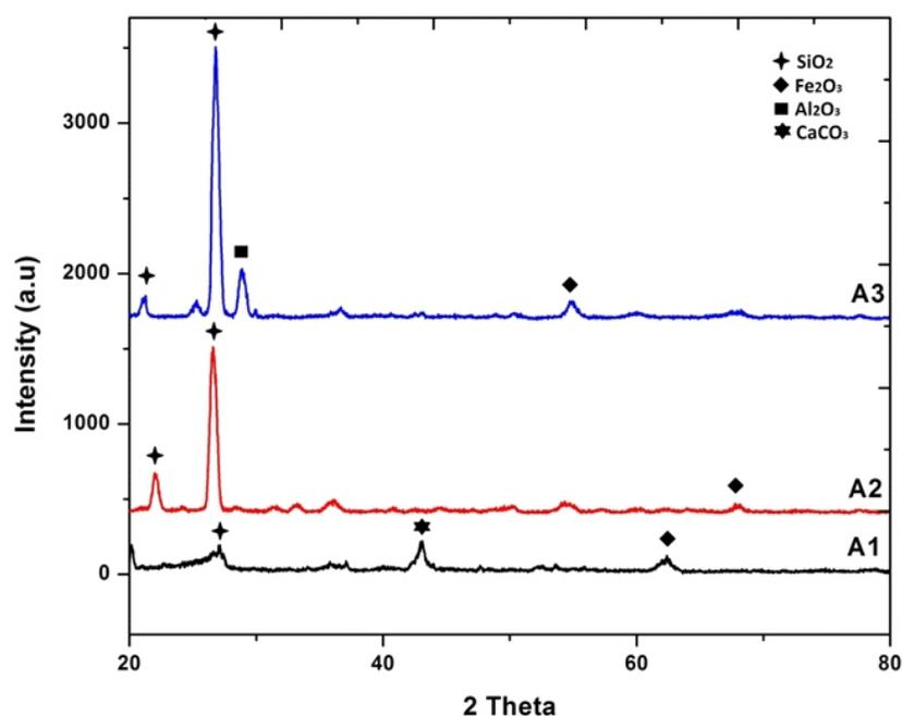
**Figure 1:** XRD pattern of the dry refractory coating
