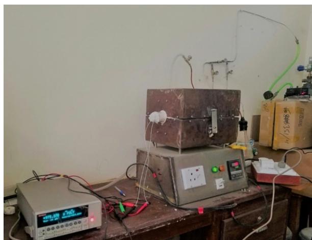
Figure 2: Gas sensor test bench for characterization of gas.
