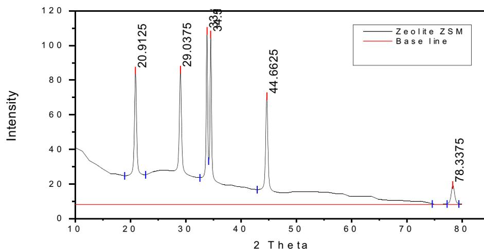
**Figure 5:** XRD Pattern of Zeolite ZSM produced from Nagarparker kaolin.
