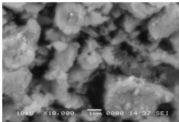
**Figure 7:** SEM of Zeolite ZSM produced from Nagarparkar kaolin (a) Resonance focus of X2500 (b) Resonance focus of x5000 and (c) Resonance of x10000
