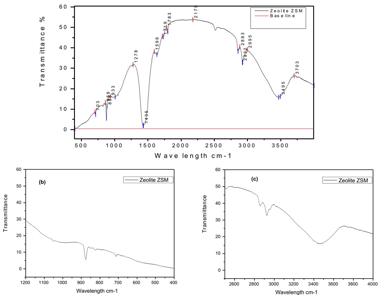
**Figure 6:** FTIR Pattern of Zeolite ZSM prepared from Nagarparker Kaolin.
