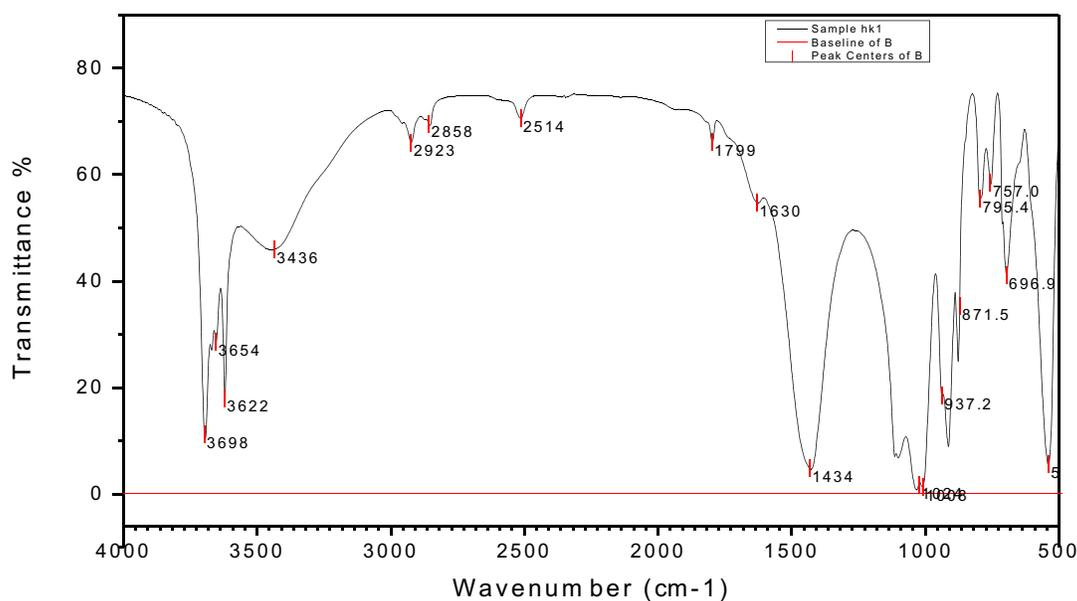
**Figure 4:** FTIR Spectrum of Nagarparker kaolin
