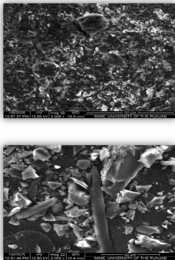
Figure 2: SEM image of Malachite green a) After adsorption b) Before adsorption
