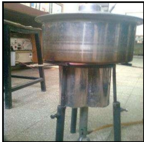
Figure 8: Deposition of carbon particles on the bottom of vessel when loading height is decreased
