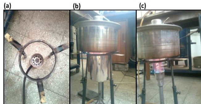
Figure 3: (a) Stand used to change loading height, (b) Burner with shield, (c) Burner without shield
